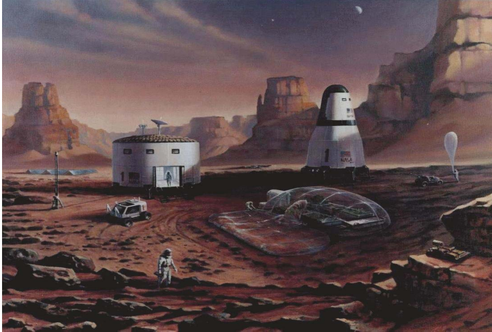
The Mars Direct plan. First an unfueled Earth Return Vehicle (ERV, right) is delivered to Mars where it manufactures its propellant from the Martian atmosphere. The crew then flies to Mars in the tuna-can-shaped hab module, which also provides living quarters, lab, and workshop for a 1.5 year Mars stay. (Artwork courtesy of Robert Murray, Pioneer Astronautics.)
