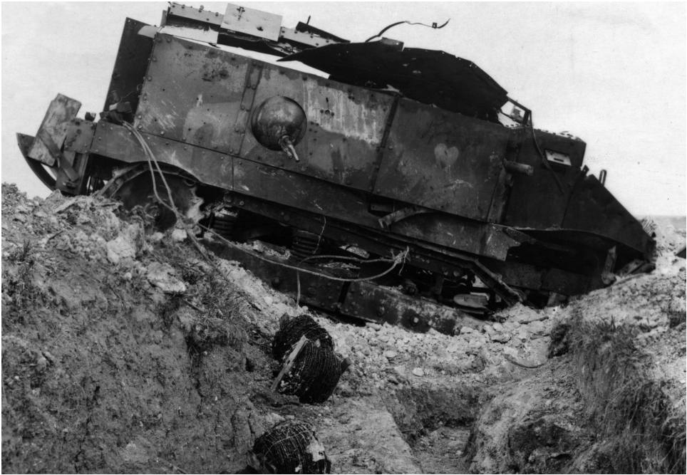
The destroyed hulk of a tank rests in a ditch, circa 1917. This Schneider CA1, the first model of French tank, bears a clear resemblance to the era's treaded farming tractors. Rolls of barbed wire appear in the foreground.
